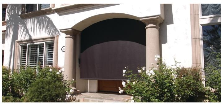
The Patio-Pro drop shade system is Accent's original drop shade allowing widths up 25 feet and heights up to 15 feet. While many upgrades have been made since its original inception in 1979, this system remains unique in its ability to be installed on inconsistent surfaces such as lattice overhangs, slanted fascia and even under eaves. This system is unlike Accent's other box and track drop shade systems.
